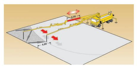
Extending the telescope increases the working surface area by 50%, the working bubble by 73%. The telescope makes it possible to pour a 4,60m wide section without movement of the boom joints.
