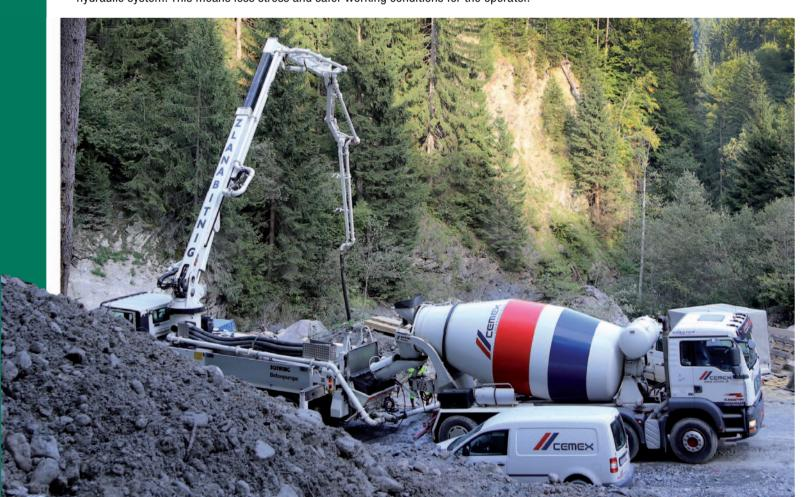
While 5-section booms in this class demand absolute concentration from their operators to avoid collision of the individual boom sections, the S 31 XT provides steering functions typical of truck-mounted concrete pumps with four-section booms.
