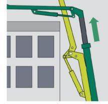
The boom can grow with the site and can thus use the horizontal working range most effectively without loosing reach.
